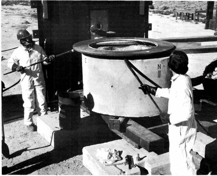
WHAT HAPPENS when molten sodium is spilled on tests simulating molten sodium spills were run with concrete is a reactor accident scenario under investigation in Advanced Reactor Research Dept. 4420. In 1980, several
